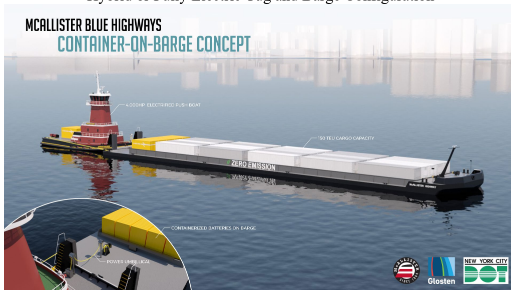
Figure 5 Hybrid or Fully Electric Tug and Barge Configuration
